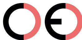
False CE Mark (too far)
